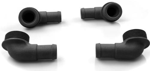
The four SLS parts that are build in the truck.
