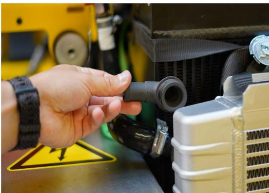
The assembled SLS part on the hybrid powertrain.
