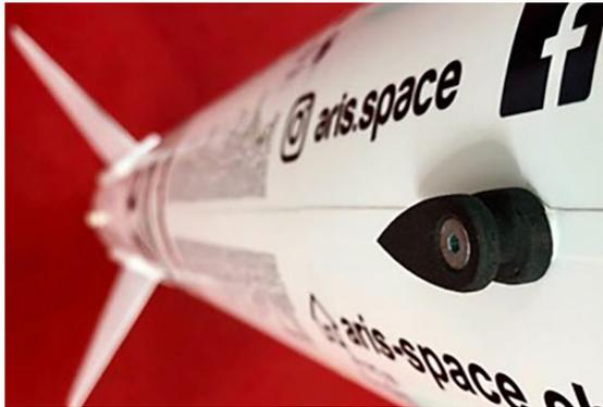
Aerodynamic and robust: The built-in launch lug is stable enough to keep the rocket in the right position during lift-off.
