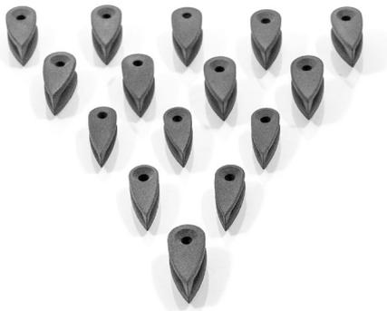
The so-called Launch Lugs were 3D-printed first in FDM, then laser sintered by Sintratec using stable polyamide 12 powder.
