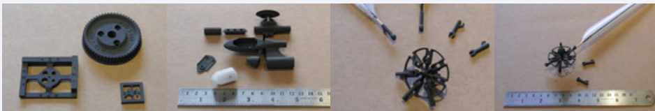
Ultrathin and light airplane modelling parts printed with the Sintratec Kit
